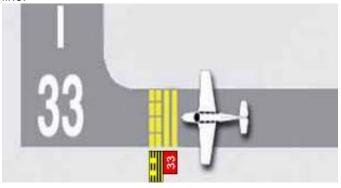
The Holding Position Sign will have a Runway Boundary Sign on the opposite side. Aircraft approaching the runway will see the red sign and must stop short of the Hold Short Line until cleared by Tower to enter the runway. Aircraft approaching from the double dashed side will see the Runway Boundary Sign and are automatically cleared to cross the line, thereby exiting the runway, unless instructed otherwise by tower.
