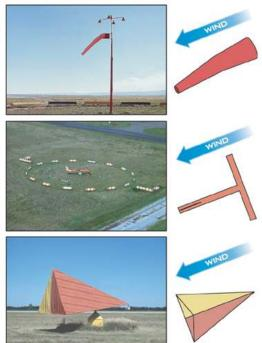
Tetrahedron – Indicates wind direction but not the intensity. It is sometimes locked in place to show the active runway.
