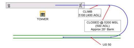
Pilots must use breakout or go-around procedures when adequate separation cannot be maintained with preceding aircraft in the traffic pattern. The preferred method to increase spacing between your aircraft and preceding aircraft in closed traffic is to extend your departure or upwind leg. Aircraft spacing on the runway must be at least 3000 feet.
