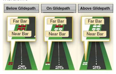
Visual Approach Slope Indicator (VASI) lights display a safe glide path to the runway. This system contains two separate bars of lights, which normally represent a 3° glide slope. When the near or lower bar is seen as white and the second or far bar, displayed as red, the aircraft is on the VASI glide path.
