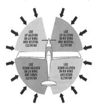
When taxiing with a quartering headwind, the wing on the upwind side will tend to be lifted by the wind unless the aileron control is held in that direction (upwind aileron UP) with the elevator NEUTRAL. This control movement will also cause the downwind aileron to be placed in the DOWN position, further reducing the tendency of the upwind wing to rise.
