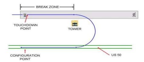
For normal landings, begin the descending 180° base turn to final when the desired aim point for the approach is 45° behind the aircraft.
