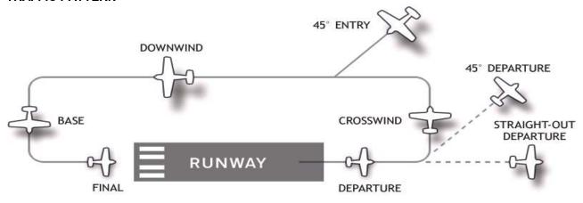
When approaching an airport for landing, the traffic pattern should be entered at a 45° angle to the downwind leg, headed toward a point abeam the midpoint of the runway to be used for landing.
