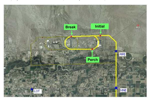
At 5,500', the standard break point for overhead pattern entries is any point within the first 2000' of the runway. ATC may direct the pilot to break at other specific locations including during the descent from Initial.
