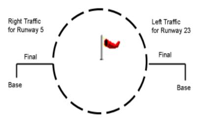
The Ls that extend from the segmented circle display the direction that the turns in the traffic pattern are made.
