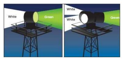
If used at airports in Class B, C, D or E airspace during the day, the beacon signifies that the ground visibility is less than 3 sm and/or the ceiling is less than 1,000 feet, conditions which prohibit VFR flight.
