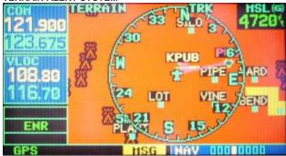
Whenever the aircraft is within 1000 feet of the surface, the terrain page turns yellow. Whenever the aircraft is within 100 feet of the surface, the page turns red. This alerts the pilot to the hazard of flying into the surface of the earth.
