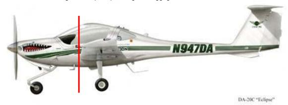
**Datum line—**an imaginary vertical plane from which all arm measurements are taken. The datum is established by the manufacturer. All moment arms and the CG range must be computed with reference to this line.
