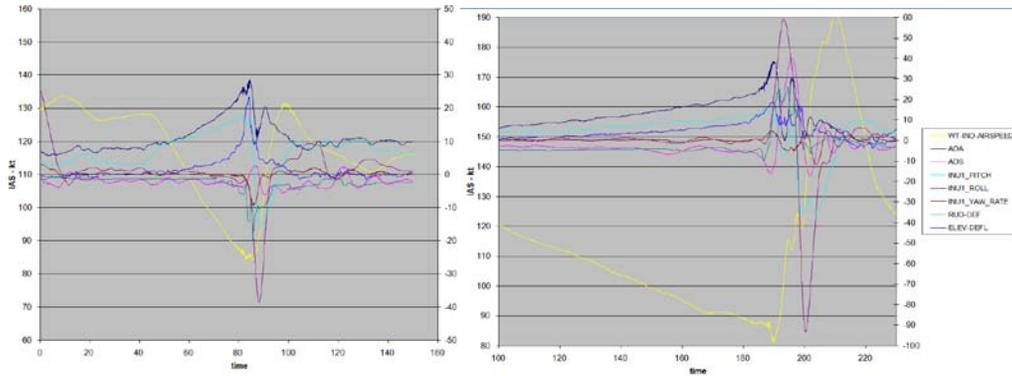
**Figure 4: 50% and 100% Flap, Power-ON Stall**
