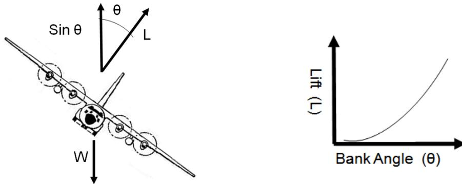
If we keep airspeed constant during the turn, the only way to increase lift is to increase angle of attack. Increasing angle of attack also increases induced drag, so power will have to be increased maintain airspeed and altitude as bank angle increases. Turn performance will be practically limited by the wing stall, power available, or aircraft g limit.
