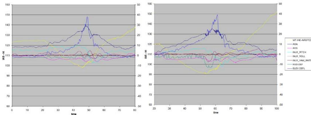
**Figure 3: 50% and 100% Flap, Power-off Stall**
