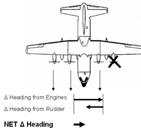
Next, let's look at the 5 degree adverse bank picture (below). The lift vector now generates a heading change in the wrong direction and induces a larger turn. Again, according to the Dash-1-1, the pilot would have to accelerate 37 knots to generate enough rudder force to counteract this turn.
