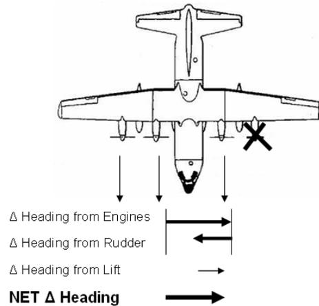
Lastly, look at an extreme scenario (below). The aircraft is in 60 degrees of bank into the dead engine. The result is a large turn in the direction the aircraft is banking.
