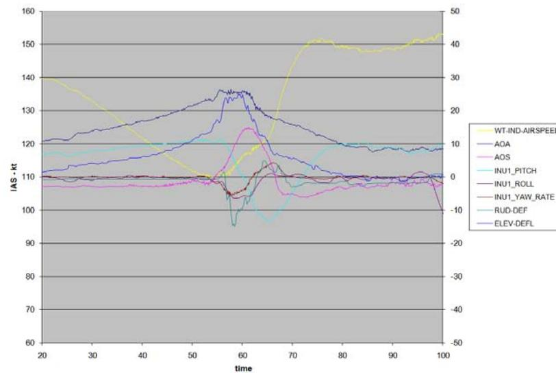
**Figure 1: 0% Flap, Power Off, Heavy Wt Stall**
