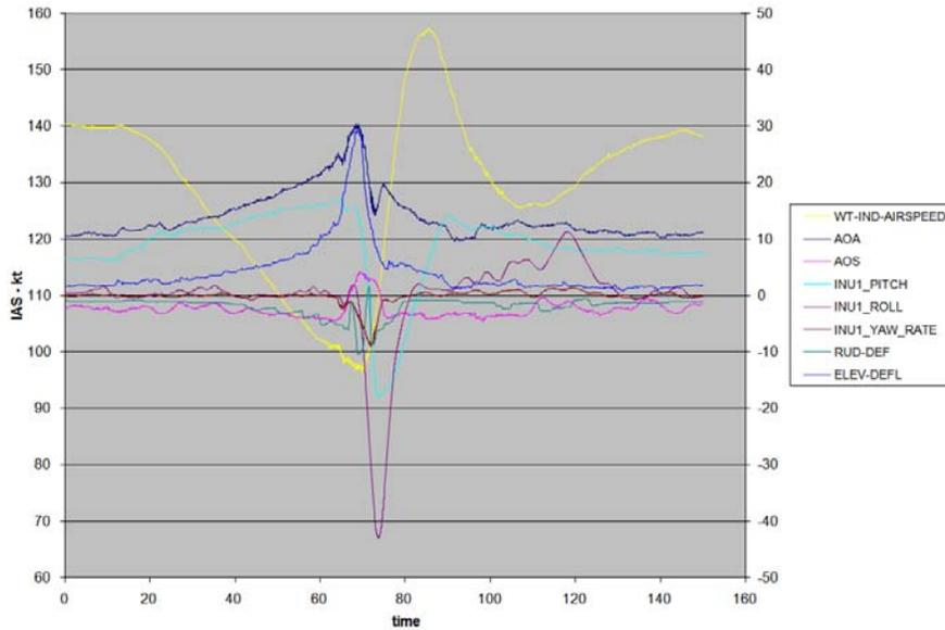
**Figure 2: 0% Flap, Power ON, Hvy wt stall**
