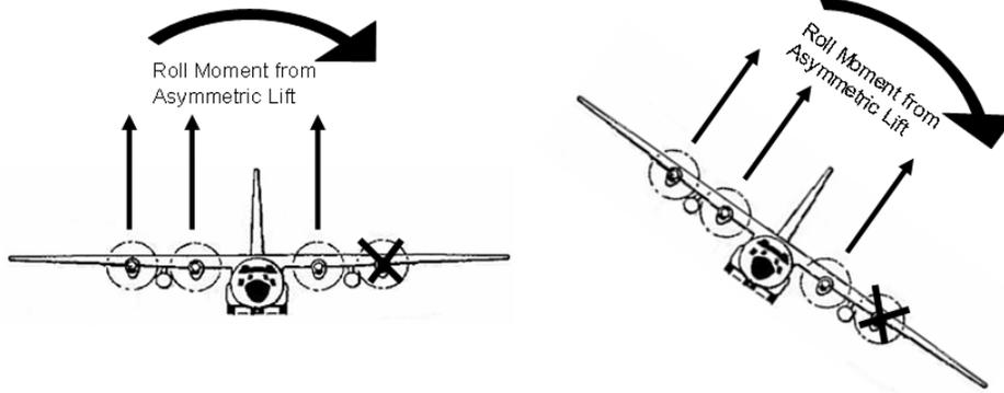
**Whether at 5 degrees of bank into the operating engines, wings level, or 45 degrees of bank into the dead engines, this asymmetric lift is not significantly different.**
