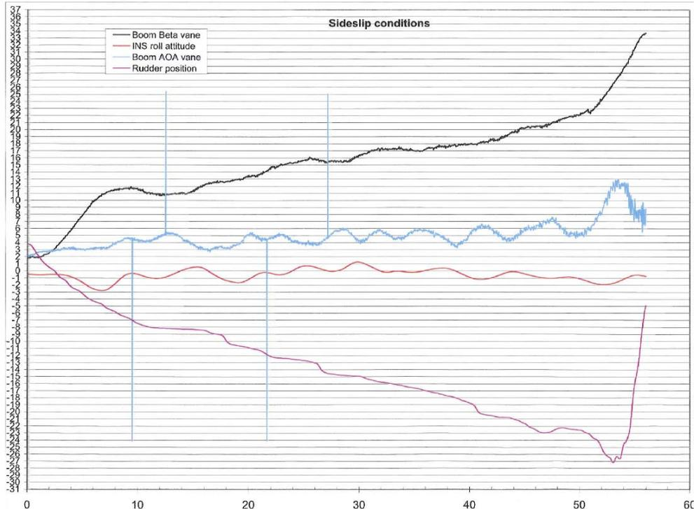
**Figure 6: Fin Stall at 23 degrees sideslip**
