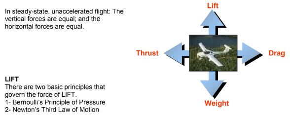
One of the principles of lift was discovered by a Swiss physicist named Bernoulli when he observed what happed to air as it passed through a tube. The principle states that: "as the velocity of a fluid or gas increases, its pressure decreases".
