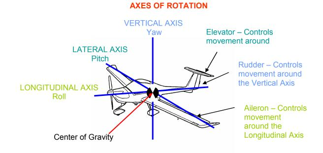
Note that in flight, the rudder is not used to turn the airplane. The primary function of the rudder is to align the fuselage with the direction of flight also known as overcoming adverse yaw. The horizontal component of lift turns the airplane.
