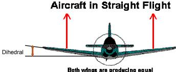
Both wings are producing equal amounts of lift. Therefore, there is no rolling moment.
