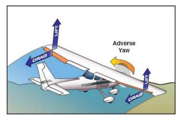
Since one wing is producing more lift than the other, a yawing force is created causing the nose of the airplane to move to the outside of the turn. This is called adverse yaw.
