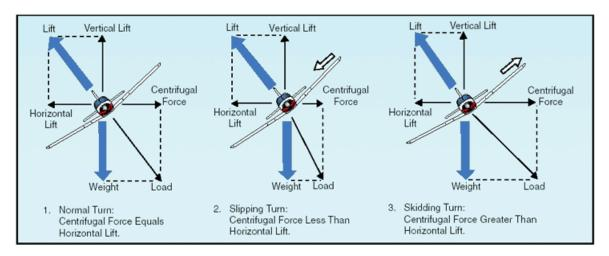
The primary flight controls are all used to perform an aerodynamically coordinated turn. Too much rudder results in a skid where the tail skids to the outside of the turn. Too little rudder results in a slip where the airplane slips to the inside of the turn.
