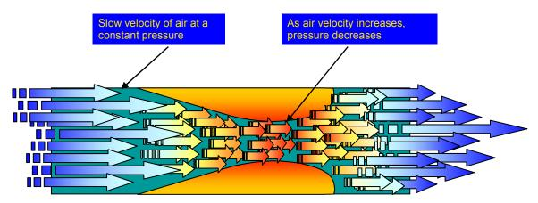
If you replace the constriction with an airfoil such as a wing, the same principle applies. As oncoming air meets at the leading edge of the airfoil, it separates. Part of the airflow goes over the top and part of the airflow goes below. Since the airflow going over the top is compressed, it must travel faster. The result is a greater decrease in air pressure above the wing.
