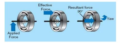
When the DA20-C1 is rotating during takeoff, the propeller plane of rotation is being forced upward which results in a turning tendency to the right. Once the propeller has stabilized in the new plane, the tendency is gone.
