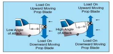
net result is that more thrust is produced on the right side of the airplane than on the left. This causes a turning tendency to the left.
