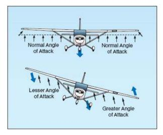
When an airplane with wing dihedral is displaced in a roll, it will immediately begin to slip in the direction of the lower wing. This creates a higher angle of attack on the low wing, which in turn increases the lift on that wing and tends to roll back to the original attitude of wings level.
