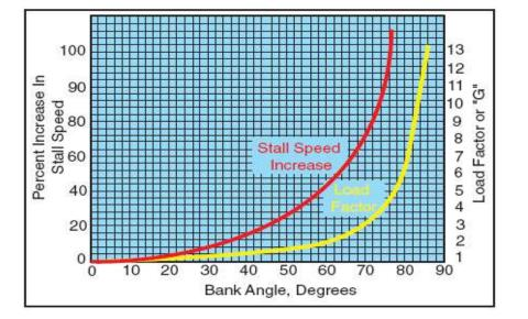
Decreasing the weight of the aircraft decreases the stall speed and increases the safety margin between normal cruise speed and stall speed. A lower weight means that less lift is required to support the aircraft. Therefore, the airplane can travel at a slower airspeed or at a lower angle of attack to create the needed amount of lift. This is desirable because it gives the pilot a larger buffer between the normal cruise speed/angle of attack and the stall speed/critical angle of attack.
