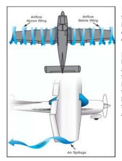
In contrast, **induced drag** is a byproduct of lift. It is drag that is incurred as a result of the production of lift. It increases with the increase in the angle of attack. It is caused by the spanwise airflow around the wing. It also decreases with velocity.
