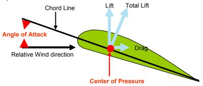
CENTER OF PRESSURE— a point along the wing chord line where lift is considered to be concentrated. For this reason, the center of pressure is commonly referred to as the center of lift.
