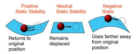
How an object responds over time (as opposed to its initial reaction) is called Dynamic Stability and can be positive, neutral, or negative.
