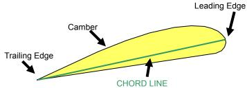
LEADING EDGE— the part of an airfoil that meets the airflow first.
