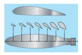
For any single revolution of the propeller, the amount of air handled depends on the blade angle, which determines how big a "bite" of air the propeller takes. Propeller slip is the difference between the geometric pitch of the propeller and its effective pitch.
