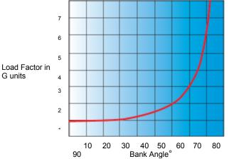
This graph shows that at bank angles of less than 45°, the load factor (and stall speed) gradually increases. At steeper bank angles, the load factor (and stall speed) increases significantly. In addition to causing an increase in stall speed, excessively high load factors can overstress airplane components.
