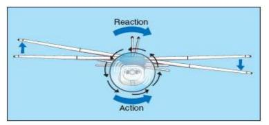
Another turning tendency is Spiraling Slipstream. The airflow behind a propeller takes on a spiraling characteristic in the direction of rotation. Since the propeller is rotating clockwise, the
