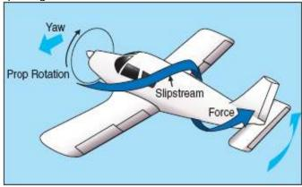
slipstream above the fuselage crosses left to right as it moves aft. This causes the vertical stabilizer to move to the right. This causes the nose of the airplane to yaw to the left. Aircraft design has counteracting forces for most of these turning tendencies, especially during cruising flight. However, at high power settings and high angles of attack, such as those used for takeoff and climb out, you will have to apply right rudder pressure to keep the airplane from turning.
