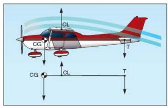
Longitudinal stability about the lateral axis is normally obtained by locating the center of gravity ahead of the center of lift, which is the point along the wing where lift is concentrated. This creates a slight nose heavy condition. To balance this condition, a tail down or nose up force is created by installation of a horizontal stabilizer with a slight negative angle of attack.
