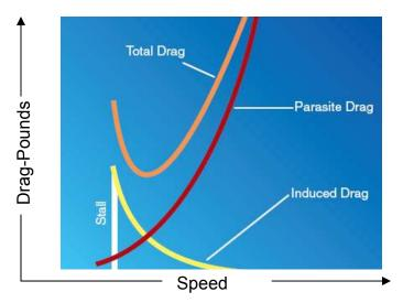
Note: Any deviation in airspeed from 73 kts, whether an increase or decrease, will result in decreased glide performance. Pilots can control the amount of lift produced in flight by changing individually, or in combination, the airplane's airspeed, angle of attack, and the wing configuration (such as lowering the flaps).
