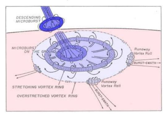
The microburst can easily exceed the performance capability of the aircraft and force the aircraft into the ground.
